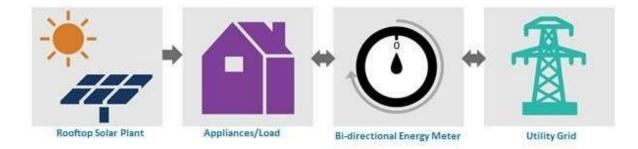
3.2 Can the RTS be installed for only captive use without being connected to Grid? Yes, the plants which are not connected to the grid are normally called behind the meter plants and MNRE subsidy is not available for such plants even for residential sector. However, it is required to follow rules and regulations specified for thispurpose by the state authorities.
